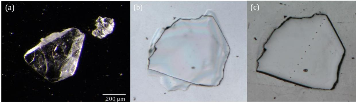
Figure 1. Photographs of an experimentally-grown quartz crystal prior to mounting (a), after mounting and polishing (b), and after analysis with EPMA (c).
