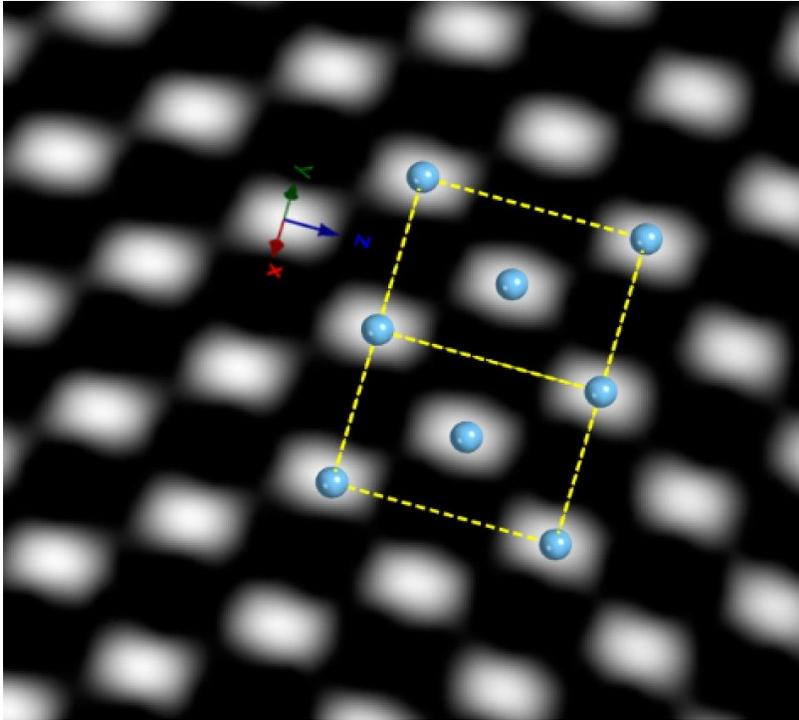
Fourier filtered high-resolution STEM micrograph from crystalline region showing the overlaid cubic TiO unit cell.
