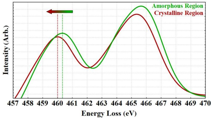
Noticeable energy loss shift in the EELS spectrum from amorphous to crystalline regions.
